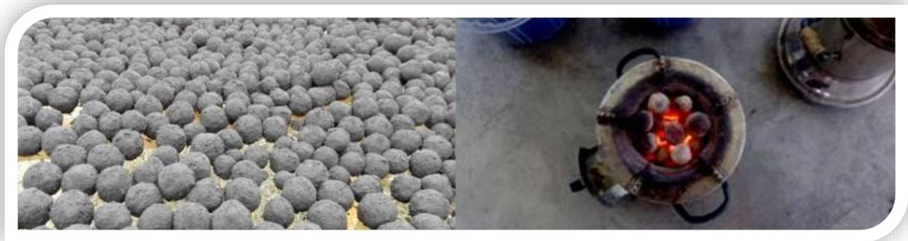
**Figure 18: Faecal char briquette (Nakuru Water and Sanitation Services Company/NAWASSCO)**
